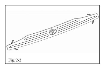
(b) Ensure all the tabs are folded so they can be accessed from the top once the protector is seated on the rear bumper (Fig. 2-2).
