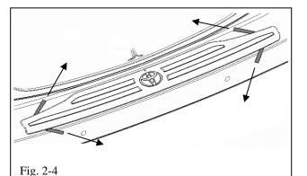
**NOTE:** Do not allow both ends of the protector to stick to the bumper before the center touches.
